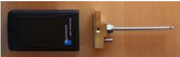
Figure 8 – New compact spectroradiometer based sensor with fine probe for use with probe locator on lamp system
